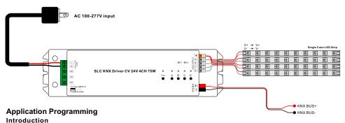
It is able to set different parameters to every output channel, and control various targets by modifying the setup of the internal parameters.
